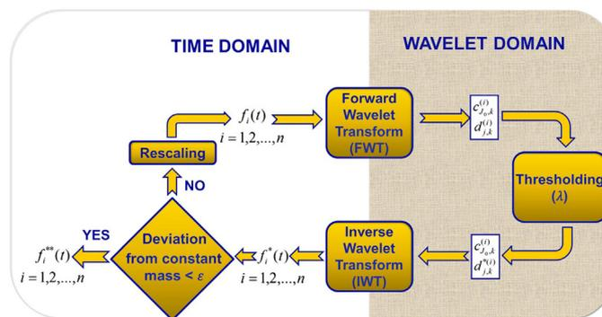
Fig. 2. Diagram of the constrained iterative wavelet smoothing (CIWS) technique.
