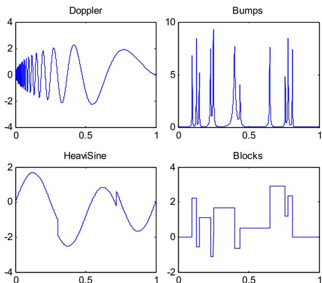
Fig. 3. Four of the set of five test functions, called *Doppler*, *Bumps*, *HeaviSine*, and *Blocks* without noise.
