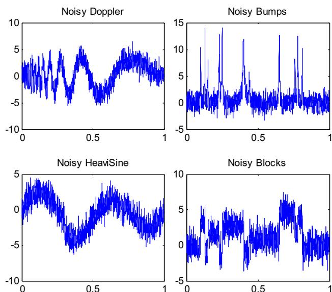
Fig. 4. Four of the set of five test functions called *Doppler*, *Bumps*, *HeaviSine*, and *Blocks* with additive white (Gaussian) noise of SNR = 15 dB.
